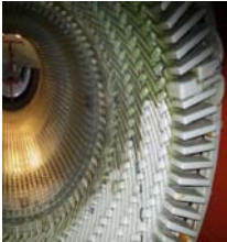
Generator part cleaned
